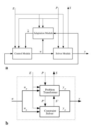
Figure 2: Adaptive Solving System Framework. The top diagram (a) shows an overview, and the bottom (b) shows an expanded view of the Solver Module.
